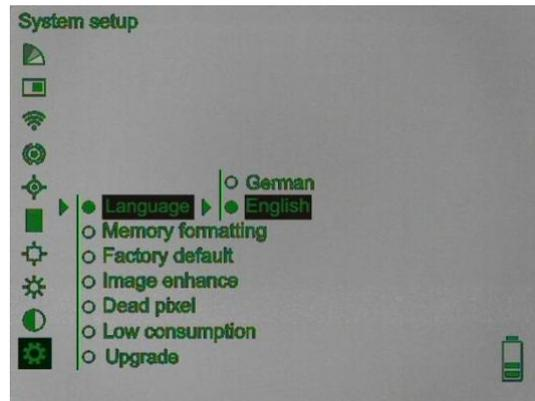
2. Memory format options, short press to select the function, turn the knob to select “Yes/No” to conduct format operation, short press the menu knob to confirm.
