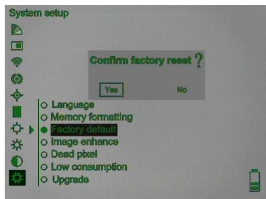
4. Image enhance option, short press to select the function, turn the knob to adjust brightness value (0~60), short press the menu knob to confirm.
